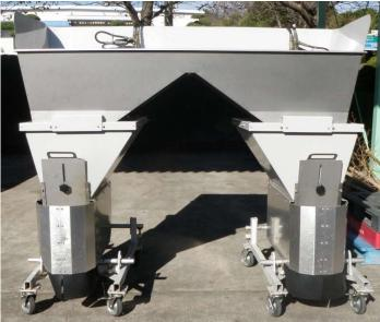
2 rows simultaneous spraying conveyor mechanism enbles smooth application It is more easy to put compost by height 200mm lower than previous model.
