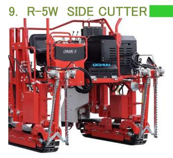
Secures the path way between tree rows 1 side, 2 sides models available Pruning attachment can be installed when single side side cutting
