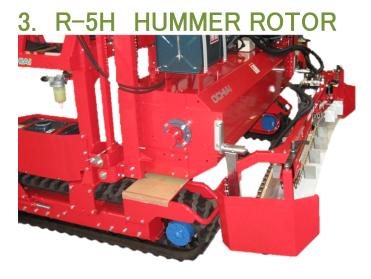
Crushing trees with hummer, and trimming with pruner. Pruning unit installed with chain
