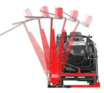
You can infinitely adjust the left and right of the angle from the operation box.
