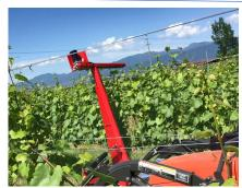
Clipper blade which is attached to L-shaped can prune the branches and leaves of the two surfaces of the top and sides.
